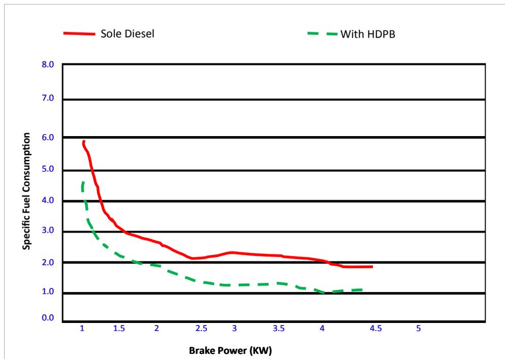
As shown in the above graph, the Specific Fuel Consumption is Low when HDPB has been used at all loads due to the proper injection of fuel in combustion chamber.
