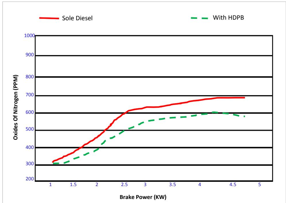
Above graph shows the variation of NOx emission with brake power of the engine. It is seen that for HDPB blend emits lower NOx level compare to standard diesel.
