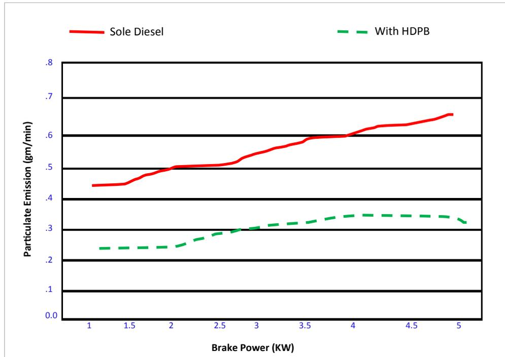
It is seen from the graph the particulate emission is Reduced when diesel blends with Hydra Diesel Power Blast.
