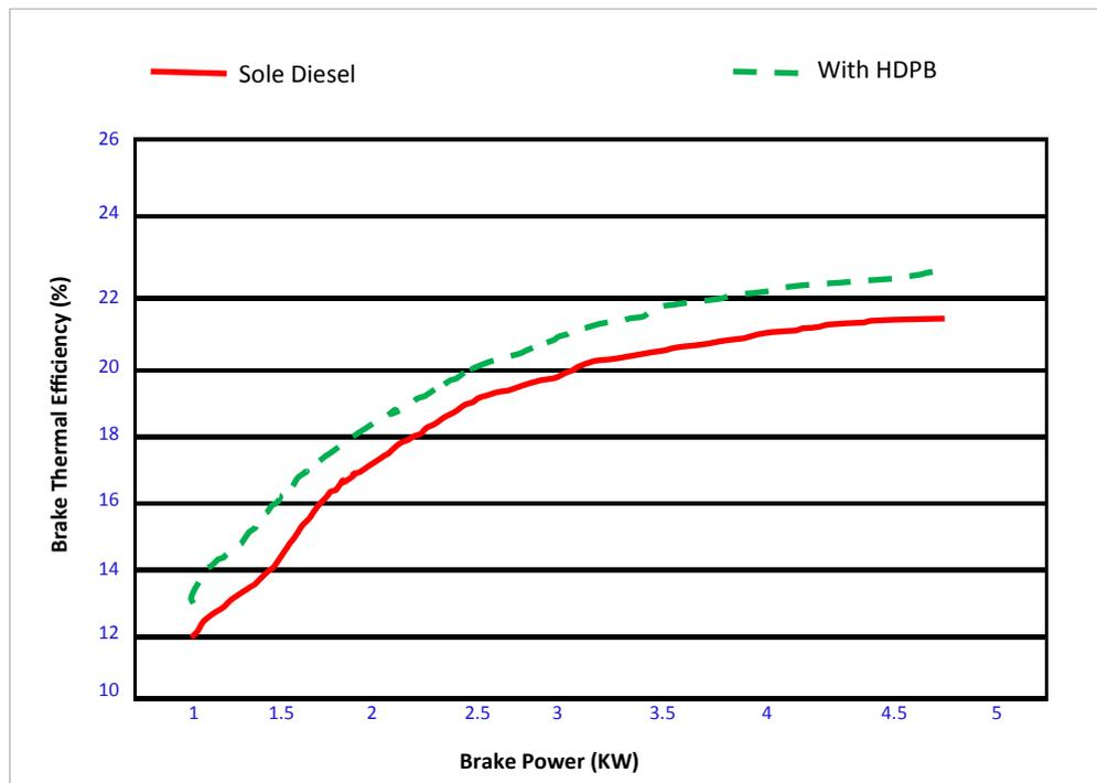
Above graph indicates the variation of Brake Thermal Efficiency with Brake Power of the engine. The Brake Thermal Efficiency at full load condition is increased with the use of HDPB and this is due to full atomization of the fuel.
