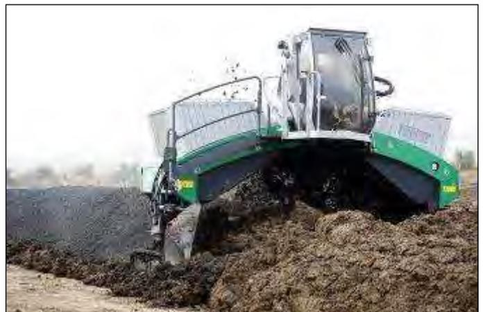
**Windrows** use periodic turning of piled polluted soil to enhance bioremediation increasing degradation activities of indigenous and/or transient hydrocarbon-oclastic bacteria present in polluted soil.
