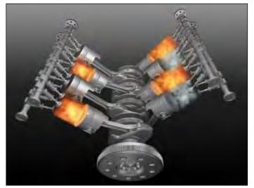
A fuel with too low of a cetane number for a particular engine will result in reduced cold-start ability, rough running, excess engine noise/vibration and reduced combustion quality.
