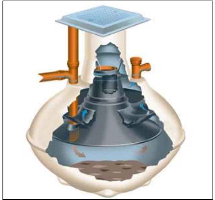
A correctly working system will break down solids, fats and grease faster, requiring less frequent emptying, will not give off unpleasant odours, and will have a cleaner liquid output to the drainage area / leech field / septic tank soak-away.
