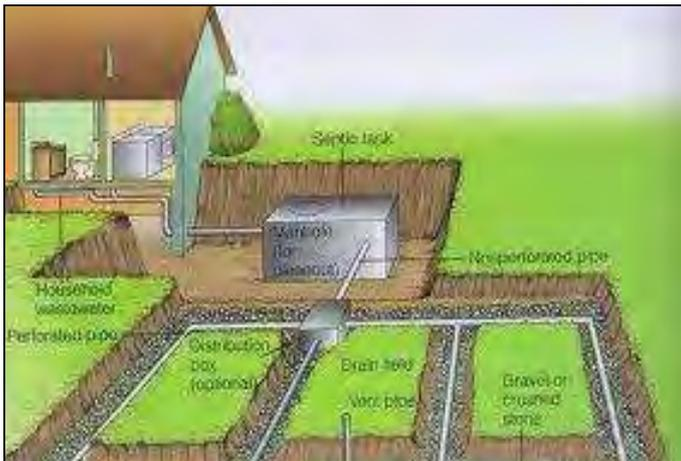
A Septic System consists of various components including: Septic Tank, Inlet wastewater pipe and a Drain field/Soak away. Waste water from the property flows into the Septic Tank directly from the drainage pipes from the sinks and toilets.
